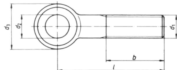
**b<sub>1</sub>** L ≤ 125mm**b<sub>2</sub>** 125mm < L ≤ 200mm
